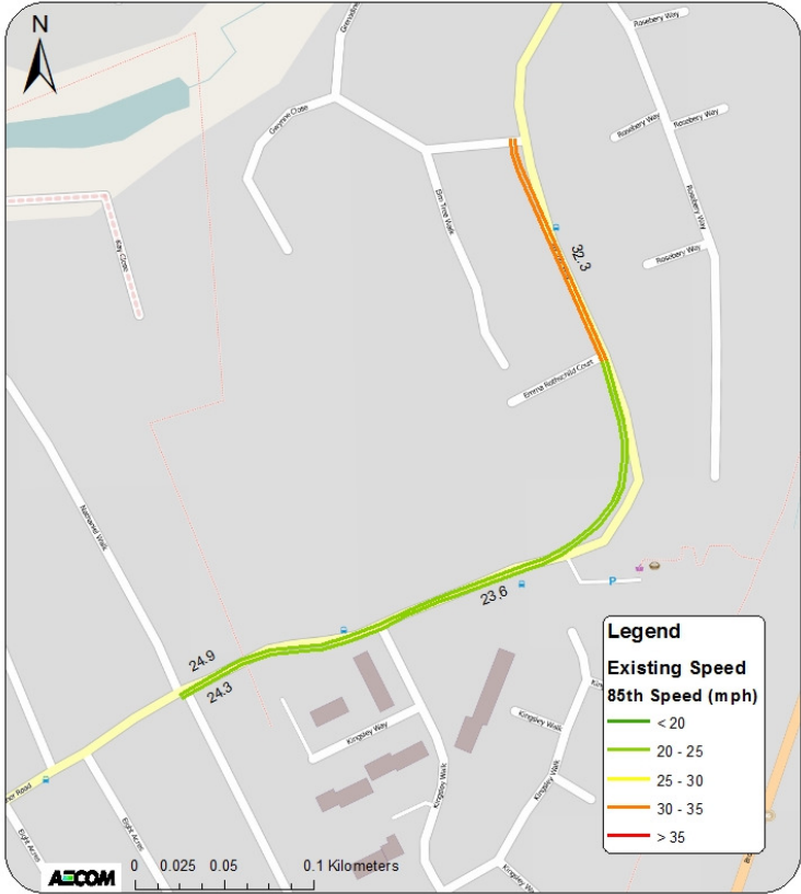
Figure 6 – 85 th percentile speeds surrounding Dundale Primary School (TrafficMaster Data for 2011)
